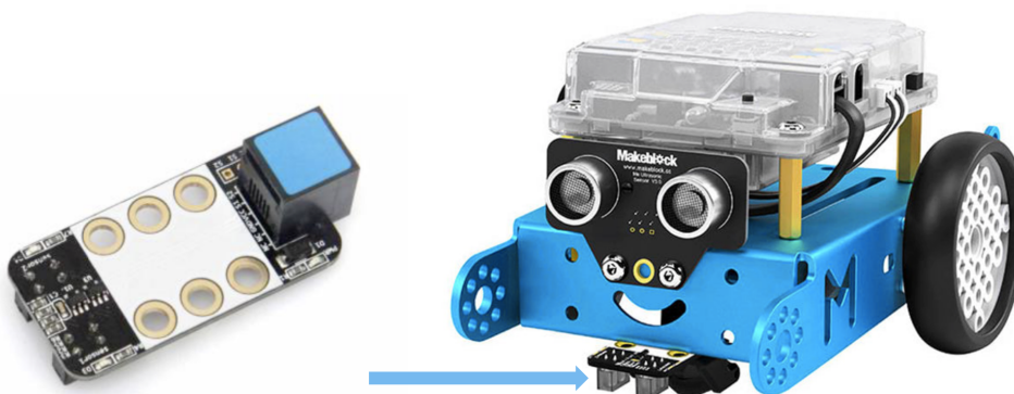
Figure: Line following sensor (left) and its location on the mBot (right)
