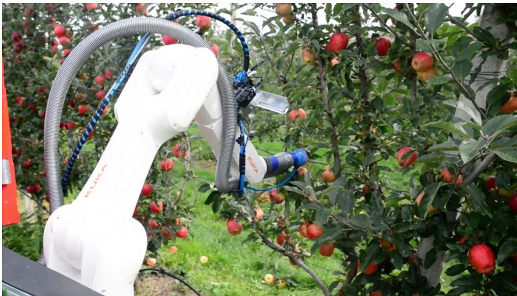
Fig. 6: Pilot project - The KUKA CropBot has mastered its first harvesting operation. It gently sucks the apples from the tree – supported by a vision system. Source: KUKA.
